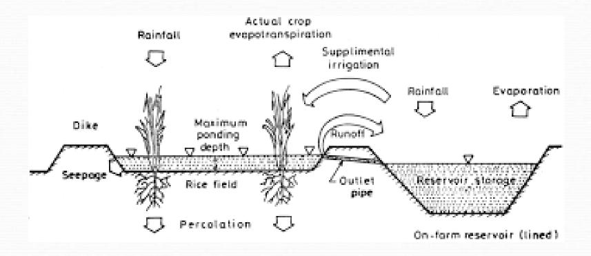
The water balance equation for a catchment is P = Q + AET + GW + DS, with all terms expressed in mm/year, where P is Precipitation, Q is Runoff, AET is actual evapotranspiration, GW is exchange with groundwater aquifer and DS is change in soil storage.
